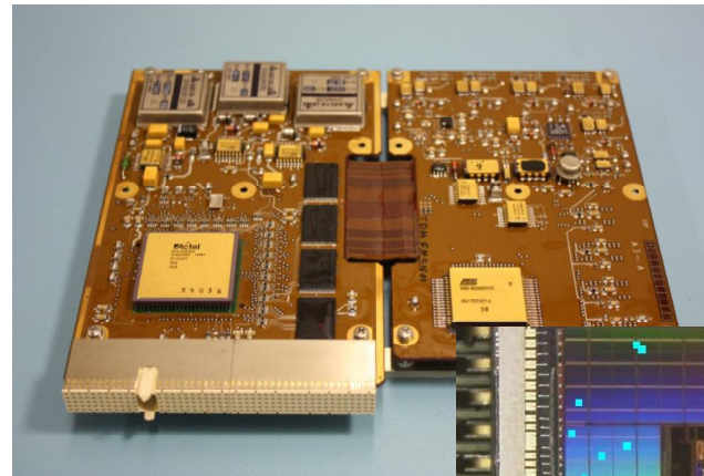
ESA Radiation Effects experiment (TDM) on board PROBA-II (low Earth orbit).
